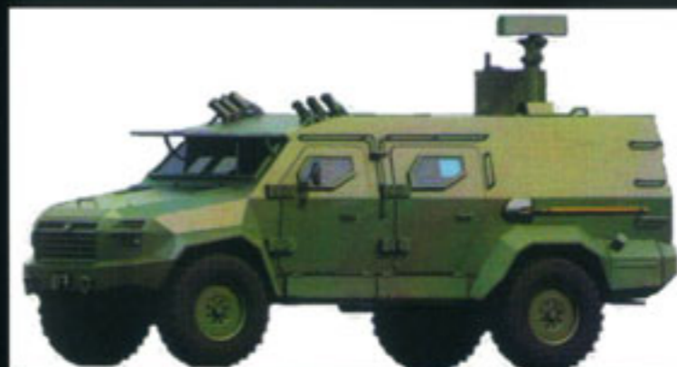
BARS-8 armored personnel carrier with "Jab" ground reconnaissance complex and "Enclave" electronic jammer
