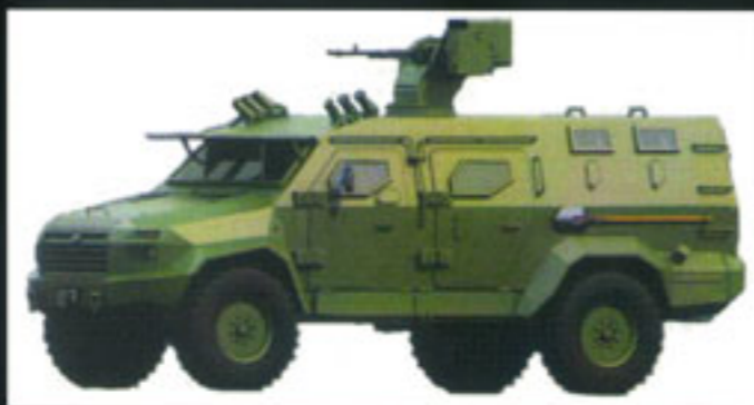
BARS-8 armored personnel carrier with "Iva" ("Willow") remote-controlled combat module
